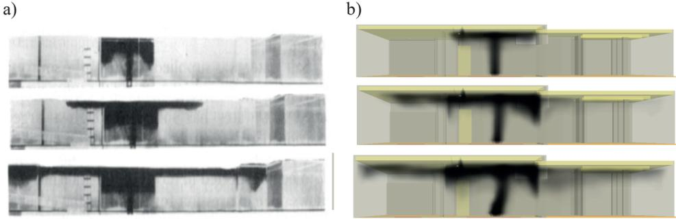
Fig. 2. Simulation of smoke spreading in a building - comparison of methods, a) analog simulation with salt water (inverted image), b) CFD computer simulation, Source: Own study based on [19]
