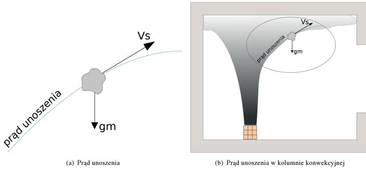
Fig. 1. Impact of gravity on the path of a moving particle. Source: Own study based on [14]
