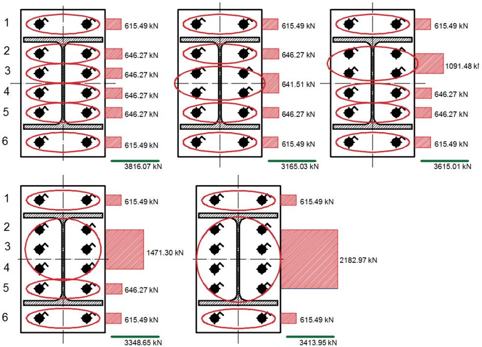
Fig. 3. Resistance of the joint at normal temperature
