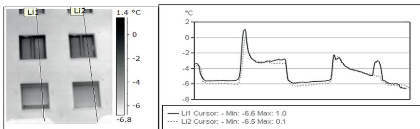
Fig. 6. Southern Poland 2012, a building made in the traditional technology after insulation. Thermogram and the analysis of window woodwork in a longitudinal wall-description in the text
