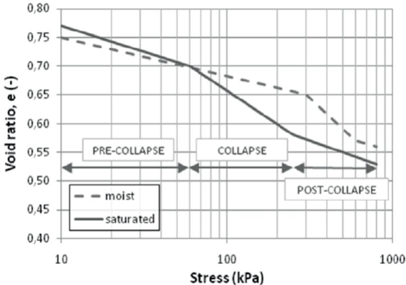
Fig. 2 Typical result of an oedometer test.
